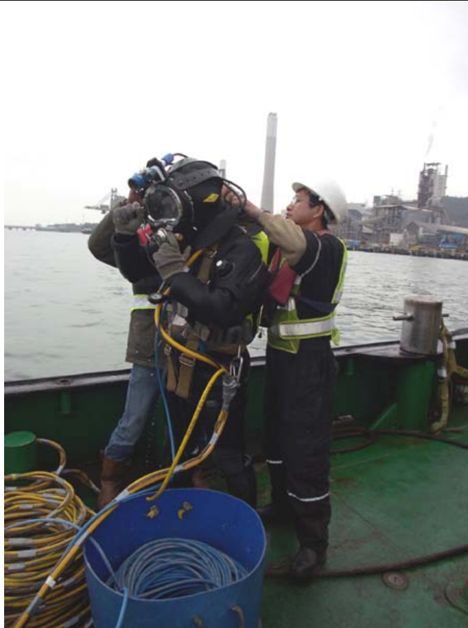
Figure 3.8 Diver Being Prepared for Diving with the Full-face Mask and the Attached Camera and Lights
